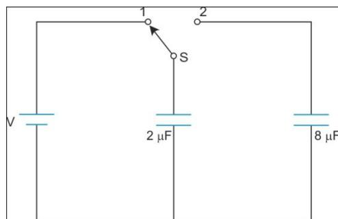
A capacitor of  $2 \mu\text{F}$  is charged as shown in the diagram. When the switch S is turned to position 2, the percentage of its stored energy dissipated is:
